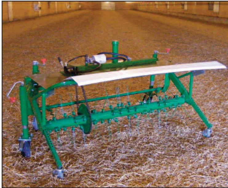
**5'8" Rotary Fork Fully Loaded with Plastic Guard Option Added**
